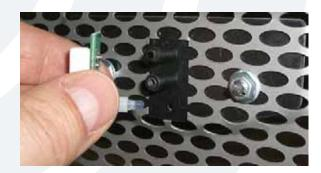
Carefully remove the led PCB assembly from the back side of the grill.
